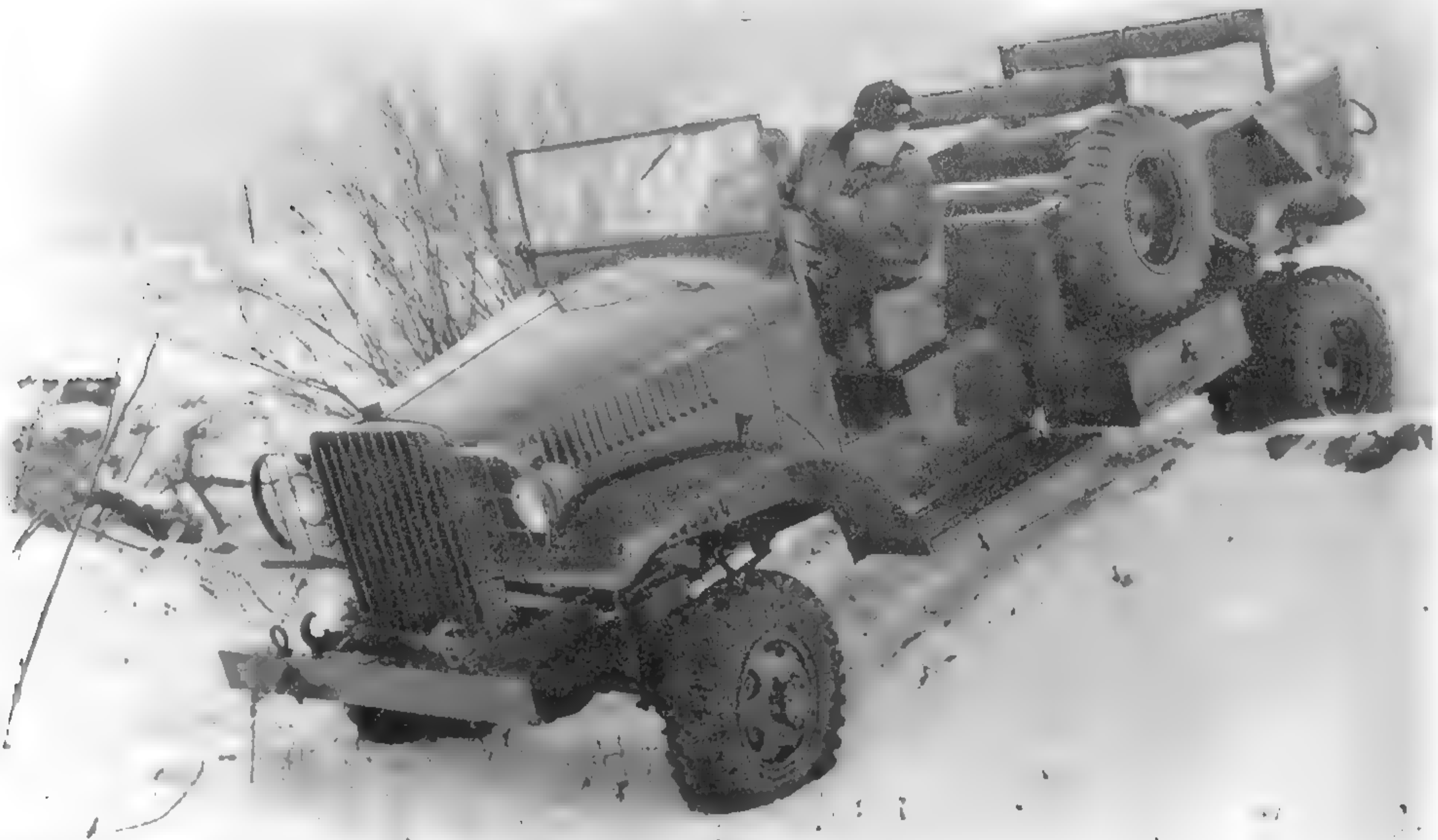
This photo of the prototype M-2-4 undergoing tests shows the general layout of these vehicles. Production units varied in details. (Photo courtesy of the Patton Museum)
